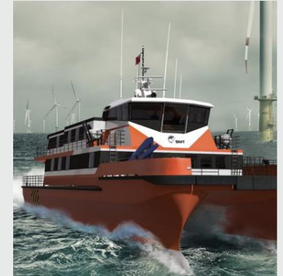
BMT designed the 36m Service Accommodation Transfer Vessel (SATV) for the Formosa 1 Offshore Wind Farm, in Taiwan.
