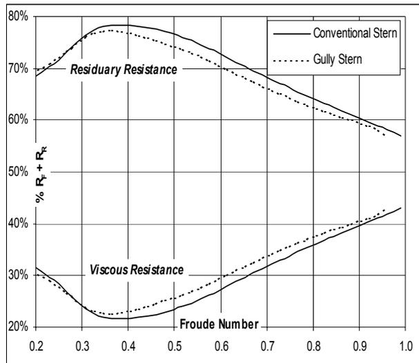
Figure 16 - %  $R_F$  & %  $R_R$  Vs  $F_N$
