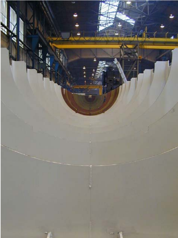
Figure 7 : Steel Jig for Construction of Floaters
