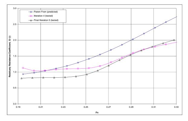
Figure 5 Final Measured Resistance Coefficients, C<sub>R</sub>
