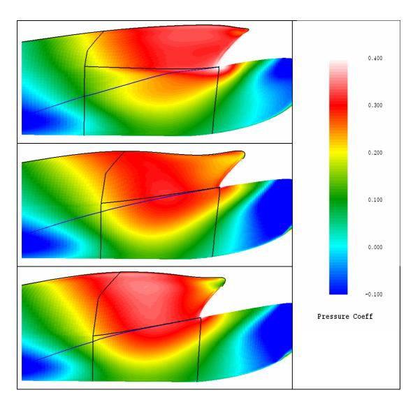
Figure 3 Pressure distribution with streamline at Vs =14 kn.
