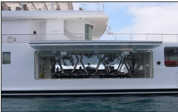
Figure 3: Tender Garage on the 138 metre Yacht, ‘Rising Sun’ – photo courtesy of www.SuperYachtTimes.com
